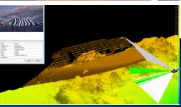
Teledyne RESON's in-house developed PDS2000 Multibeam is designed to efficiently create high quality, fast results - whether it is for multibeam surveys, singlebeam surveys, construction or dredging works.
